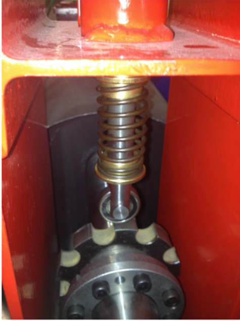
Fig. 14. Localized fault emulator.
