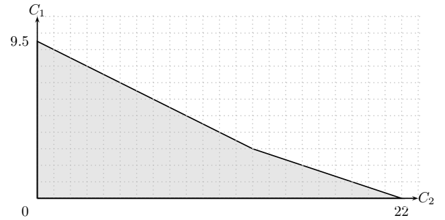
Figure 2. Example of the representation of the \mathbb{C} -space of a system composed of 2 tasks, with T_1 = D_1 = 9.5 and T_2 = D_2 = 22
