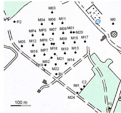
Fig. 2. Drilled boreholes on the HES cover a grid of 210 m × 210 m
