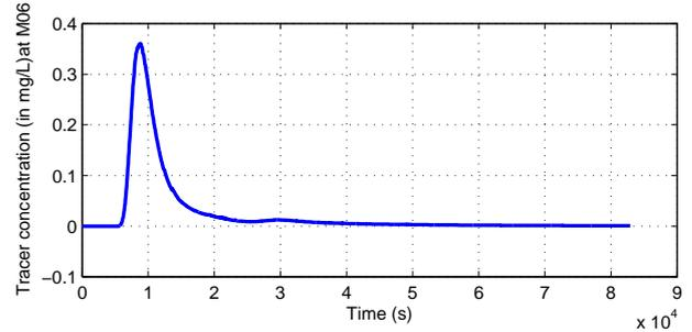
Fig. 8. Concentration estimation of a marker at M06 when injected at M07 (50 m away)
