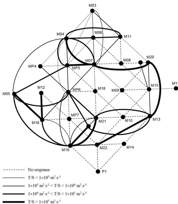
Fig. 10. Hydraulic diffusivity ( $T/S$ ) values interpreted from cross-borehole slug-tests with the method of Audouin and Bodin (2008)
