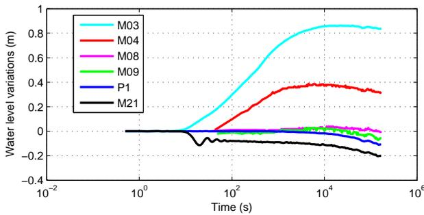
Fig. 6. M06-M22 dipole test: water level variations at 6 observation wells
