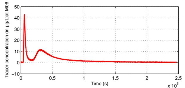
Fig. 9. Concentration estimation of a marker at M06 when injected at M04 (50 m away)
