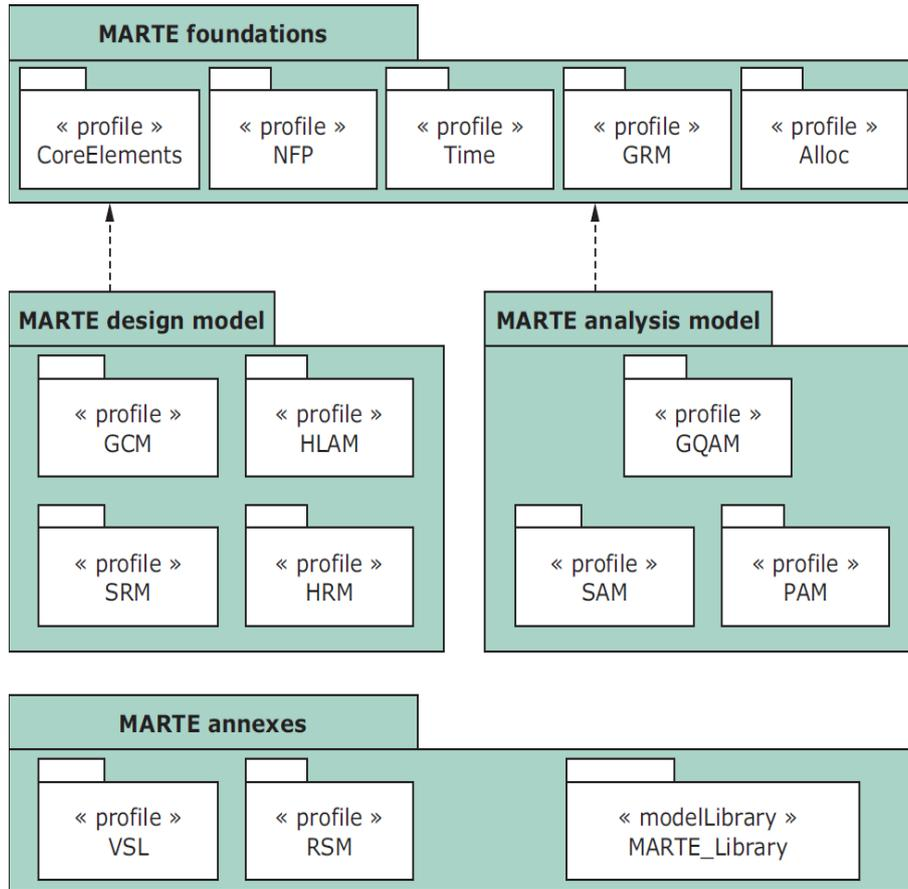
Figure 4.9: Architecture of the MARTE profile [OMG09]
