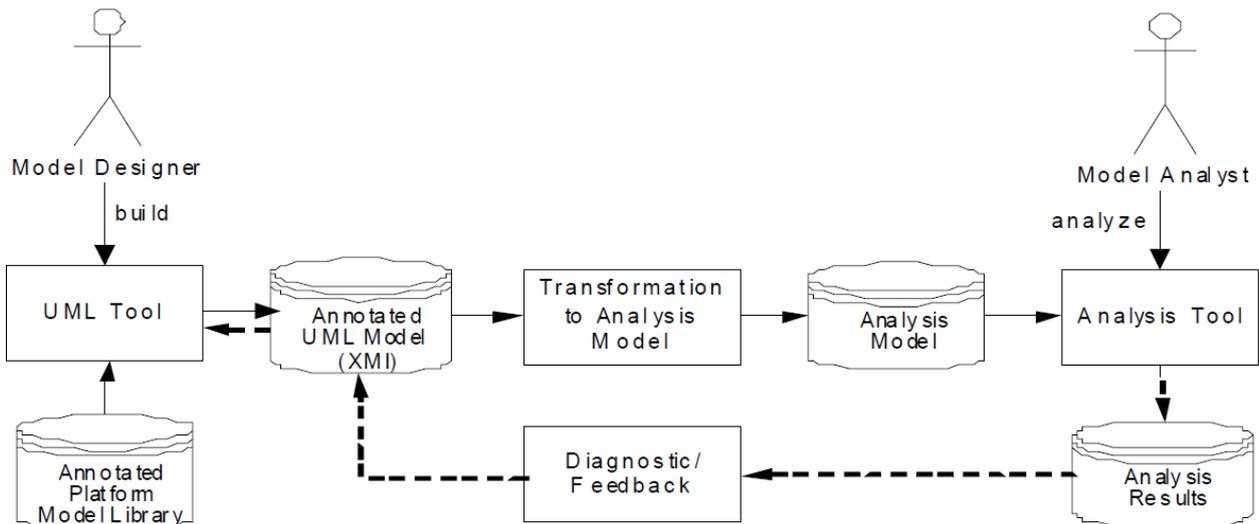
Figure 5.5: A tool chain for carrying out the analysis of a model [OMG09]
