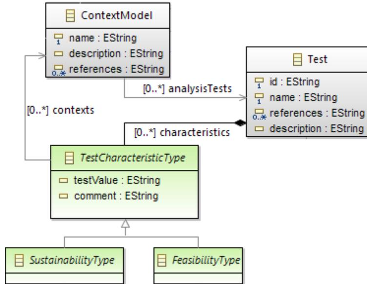
Figure 7.4: Test class, its interactions and its properties
