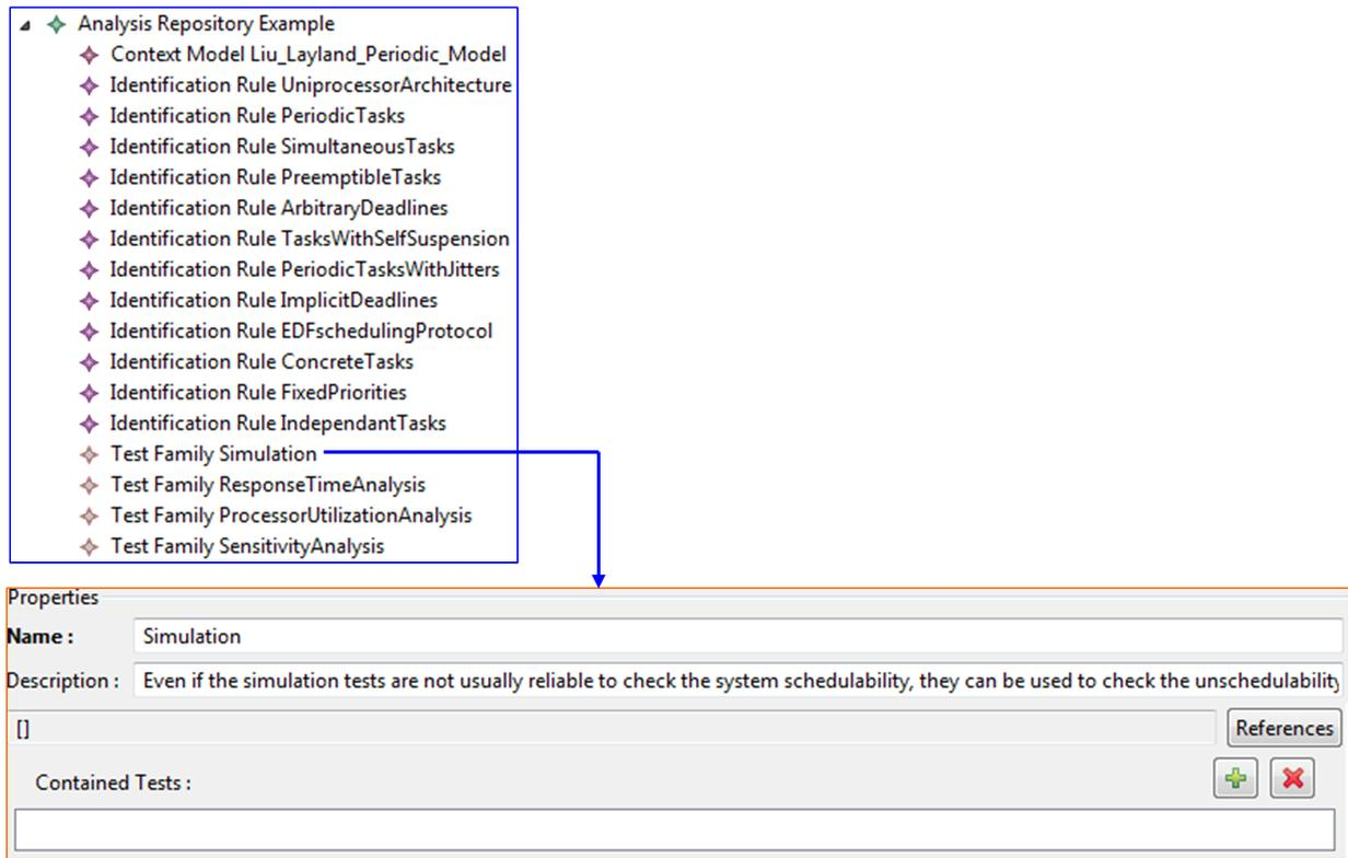
Figure 7.11: Simulation test family and its properties
