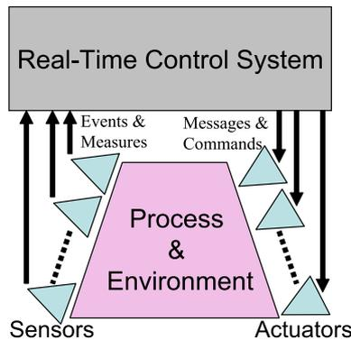
Figure 2.1: A generic architecture of a real-time system
