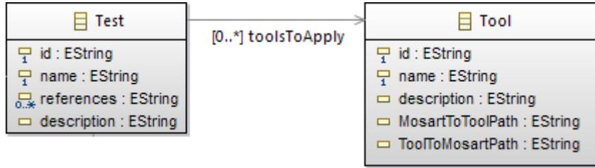
Figure 7.6: Tool class, its interactions and its properties
