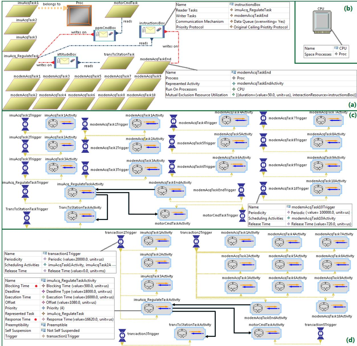
Figure 8.15: Parts (a), (b) and (c) represent an extract from the MoSaRT model obtained via the transformation process from AADL model. Part (d) represents an extract from the refined model [The refinement is realized by a transformation from MoSaRT to MoSaRT]
