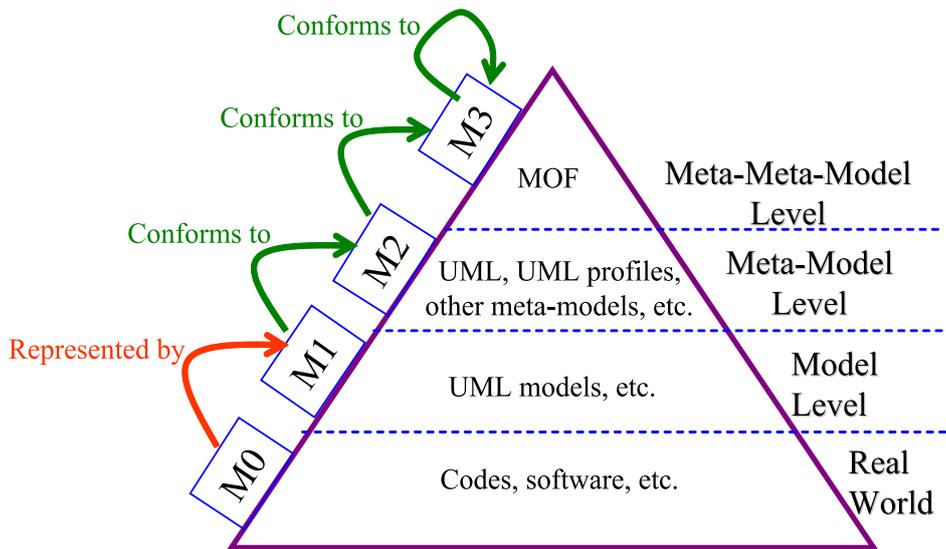
Figure 4.3: Four-layered architecture of MDA [BB02]
