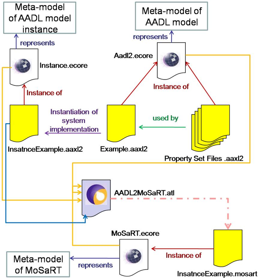
Figure 8.14: Architecture of the transformation process between AADL and MoSaRT
