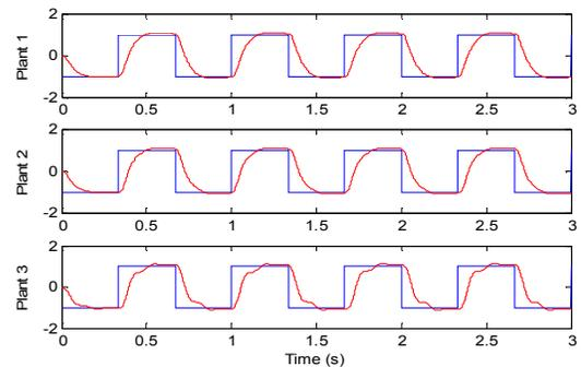
Figure 12. Control performance of three plant with EDfbs\_eg (case 3)
