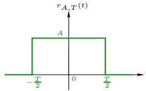
FIGURE 3.1 – Signal  $r_{A,T}(t)$
